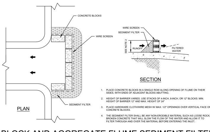
BLOCK AND AGGREGATE FLUME SEDIMENT FILTER BS
