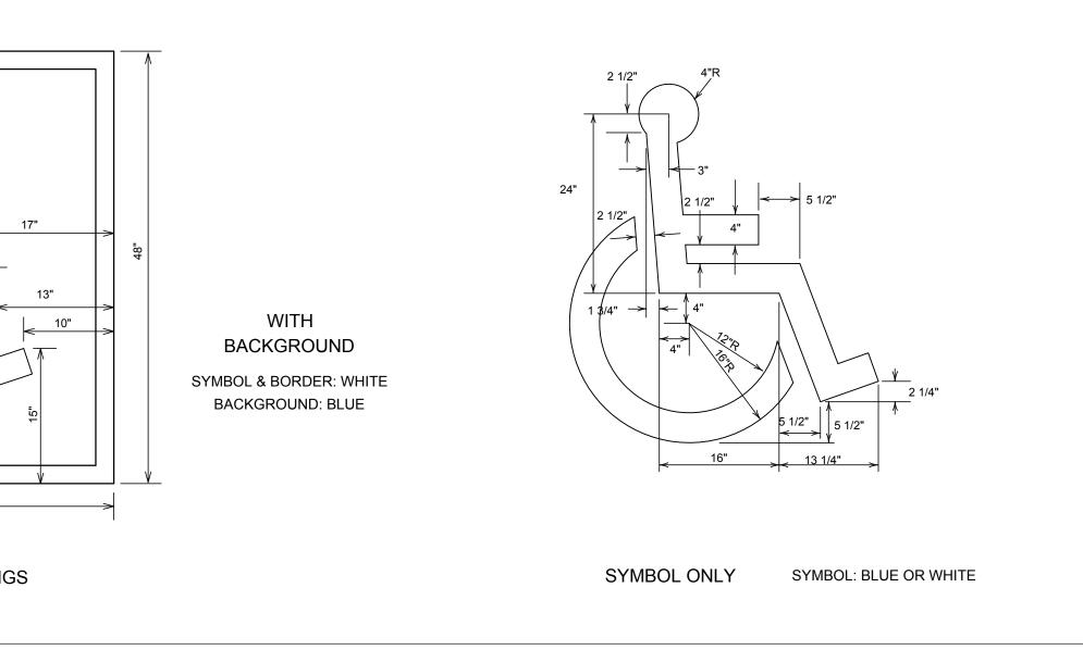
VIOLATORS SUBJECT TO FINE AND TOWING, THE BOTTOM -OF THIS SIGN SHALL BE 48" MINIMUM AND 80" MAXIMUM ABOVE GROUND AND NO MORE THAN 8" BELOW ACCESSIBLE PARKING SIGN
