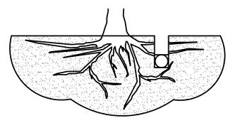
OPEN TRENCHING MAY BE USED IF EXPOSED TREE ROOTS DO NOT EXCEED 3" OR ROOTS CAN BE BENT BACK.
