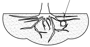
TUNNEL TO MINIMIZE ROOT DAMAGE (TOP) AS OPPOSED TO SURFACE-DUG TRENCHES IN ROOT PROTECTION ZONE WHEN THE 5' MINIMUM DISTANCE FROM TRUNK CAN NOT BE ACHIEVED.
